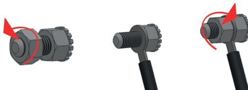
Figure 10. Connecting the unit to an electrical equalizing system.
