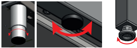
Figure 3. Leveling the device
