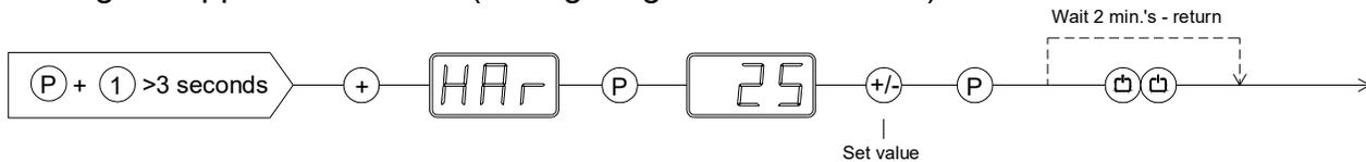
Setting the lower alarm value (setting range  $-35^{\circ}\text{C}$  to  $+25^{\circ}\text{C}$ ):
